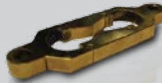
Ductility Mould (A-440/M)
