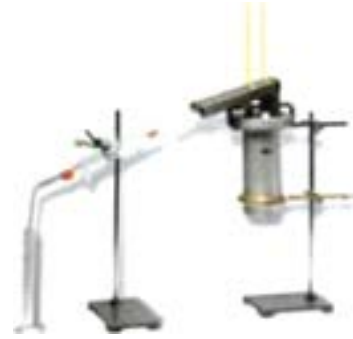
Emulsion - Distillation Unit (A-450)
