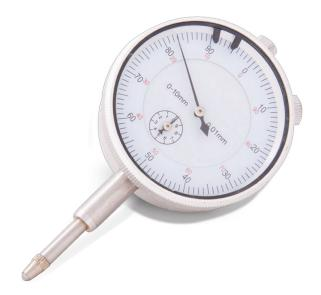
• Dial gauges serve a crucial purpose in the realm of measurements, as they are adept at quantifying not only vertical but also horizontal deformations. Their utility spans across a diverse array of tests, encompassing a wide spectrum of industries and applications. By facilitating the precise assessment of both vertical and horizontal shifts or distortions, these gauges contribute indispensably to ensuring accurate data collection and informed decision-making within various testing scenarios.
