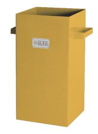
• Used to determine the consistency of fresh concrete by determining its degree of compactability.
