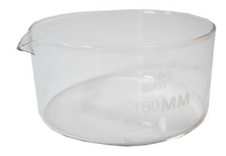
A crystallizing dish in engineering testing laboratories is used for evaporating solvents and facilitating the
