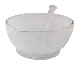
A glass mortar and pestle in engineering testing laboratories are used for grinding and mixing materials, particularly for substances that may react with porcelain or other materials. The smooth surface of glass ensures no contamination and is ideal for preparing fine powders or combining chemicals in precise quantities for testing.
