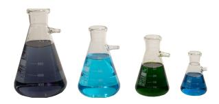
• A filtering flask in engineering testing laboratories is used to hold liquids during filtration processes. It is typically used with a vacuum pump to create suction, which speeds up the filtration of liquids through a filter paper, ensuring the separation of solids from liquids in various chemical or material testing procedures.
