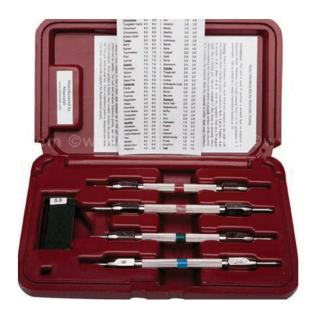
A Moh's hardness kit in engineering testing laboratories is used to measure the hardness of materials, such as minerals or rocks, based on their ability to resist scratching. The kit includes a set of reference minerals with known hardness values, allowing accurate determination of material hardness for geological or material testing.
