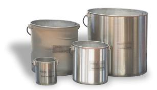
A unit weight measure in engineering testing laboratories is used to determine the unit weight or density
