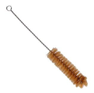
• A tube brush in engineering testing laboratories is used for cleaning narrow, cylindrical surfaces such as test tubes, pipes, or small containers. It helps remove debris, residue, or contaminants, ensuring accurate and reliable testing and preventing cross-contamination.
