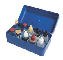
• A water quality test kit in engineering testing laboratories is used to assess various parameters of water, such as pH, turbidity, dissolved oxygen, and chemical contaminants. It helps ensure that water meets environmental and regulatory standards for quality before use in construction or other processes.
