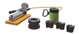
Used to determine the pullout strength of hardened concrete by measuring the force required to pull an anchor steel rebar from a concrete test specimen or structure. The insert or rebar is either cast into fresh concrete or installed in hardened concrete.
